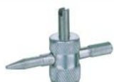
VCT-10 Core screwdriver, rethreads inside and outside part of stems, extracting damaged cores and deflating tires
